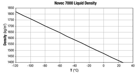
Liquid Density  $[kg/m^3] = 1472.6 - 2.880 \cdot T(^{\circ}C)$
